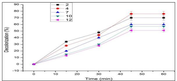
Fig. 4. Effect of different pH on decolorization of Remazol Black B by crude laccase.
