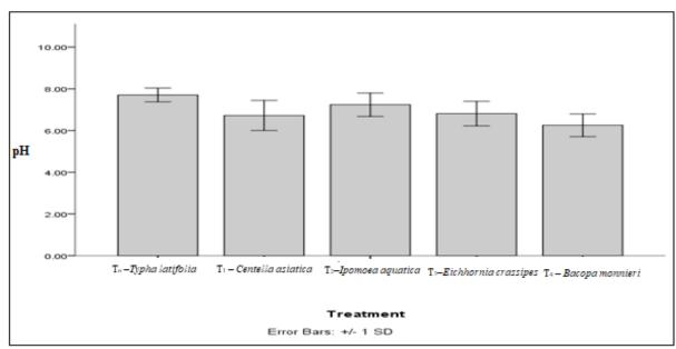
Fig. 2. Potential of the hydrogen after 15 days of growing of the five treatment plant species.
