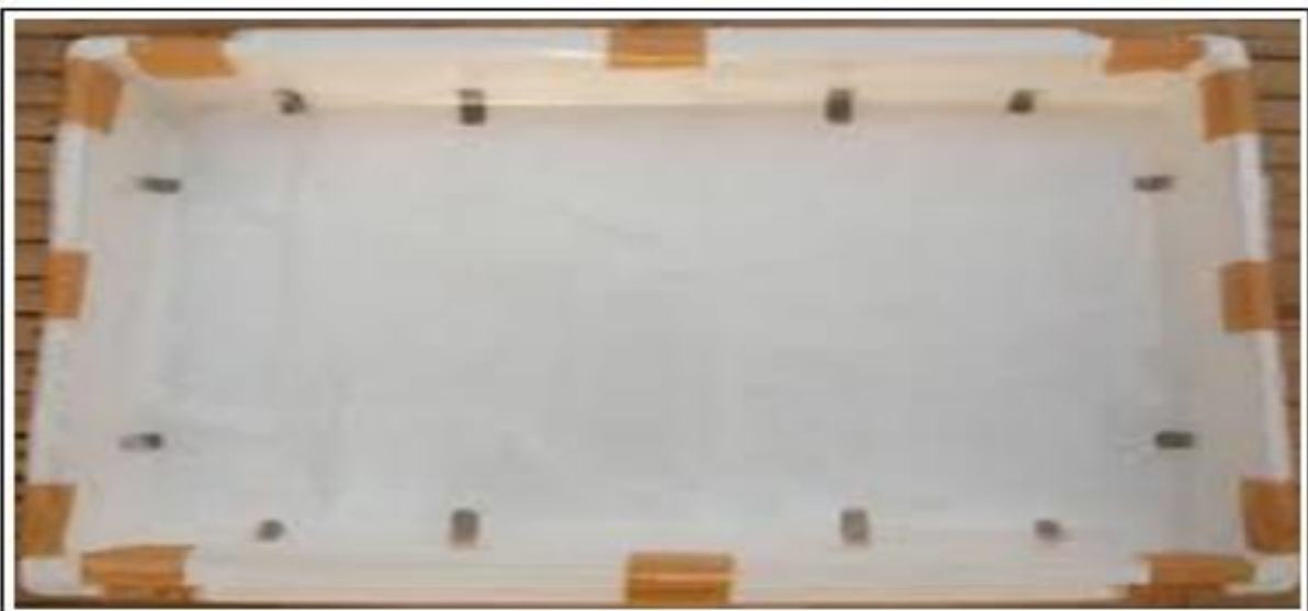
Fig. 2. Plastic bag as the liner of the bottom half on the box.
