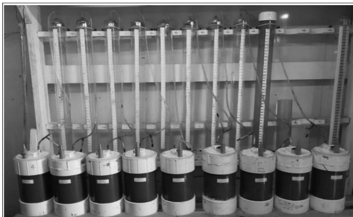
Fig. 1. Experimental set-up for the Anaerobic Digestion of biomass.
