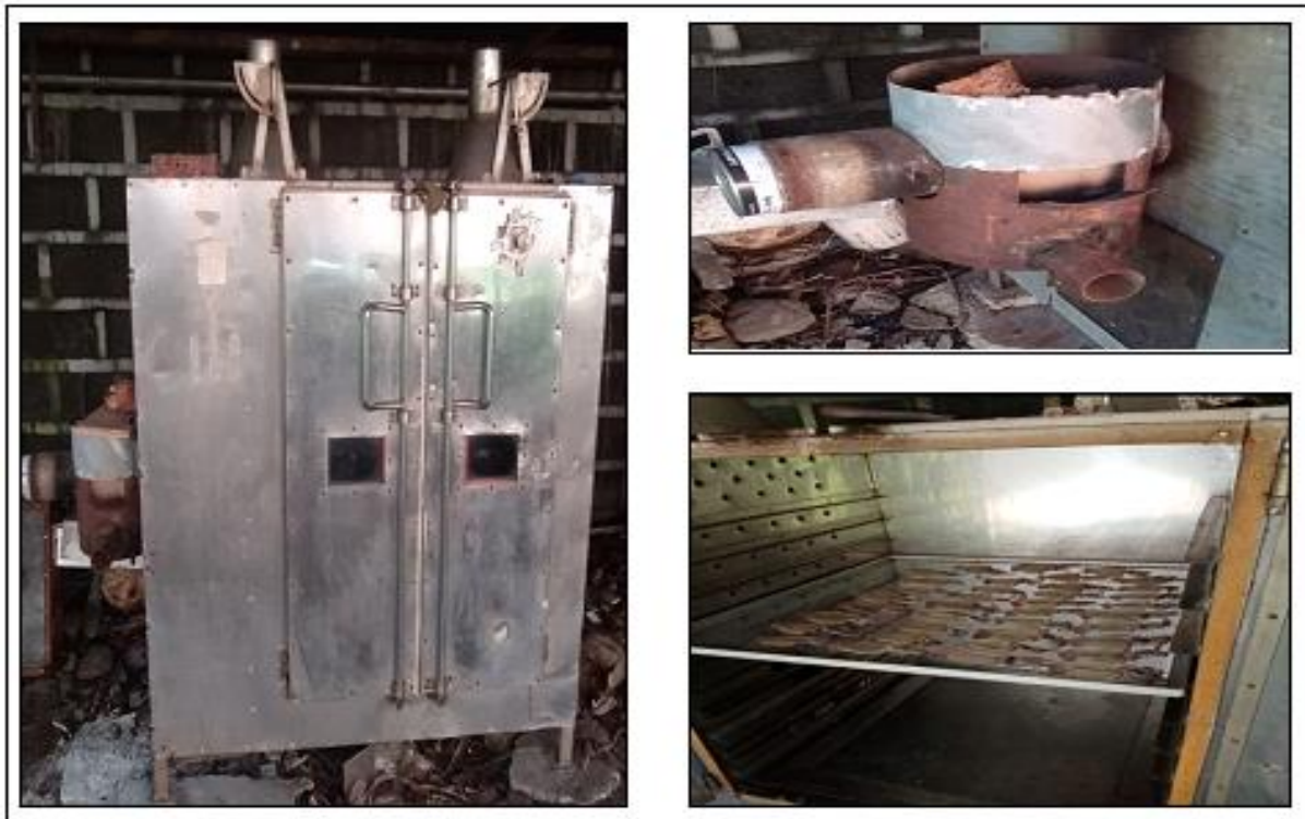
Fig. 4. Actual design of the fabricated dryer.
