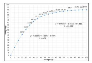
**Fig. 4.** Represents the best fit curve for relationship between percent length of lining and reduction of water-loss/salvation of lost water.
