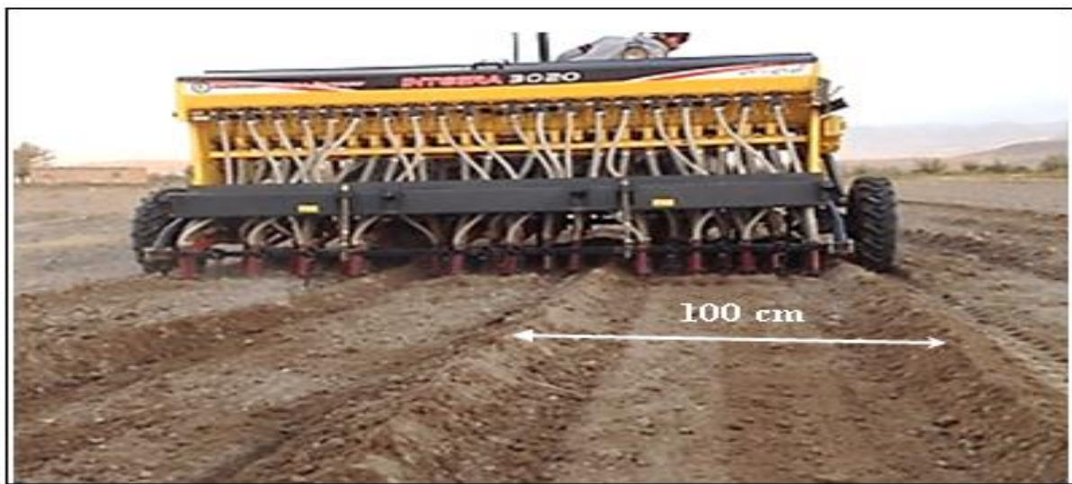
Fig. 3. The 20-Row drill planter which create three furrows with 100 cm width.
