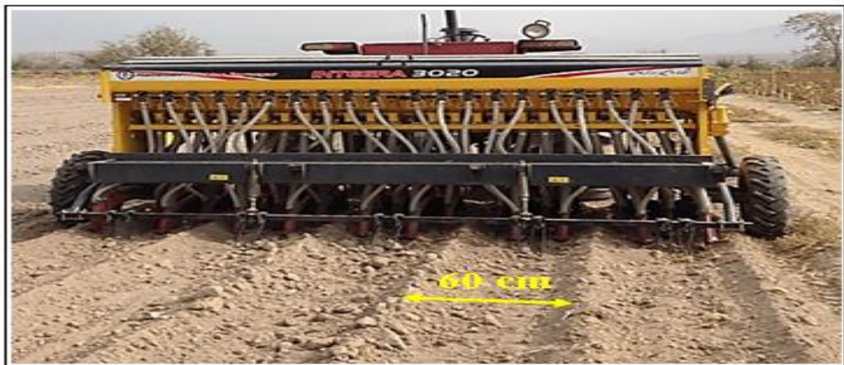
Fig. 2. The 20-Row drill planters which create five furrows with 60 cm width.
