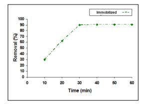
**Fig. 3.** Effect of time of the removal of phenolic compounds from wastewater by immobilized laccase.
