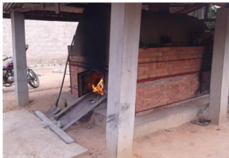
Figure 3. CISSE LABEL type incinerator in Africa.
