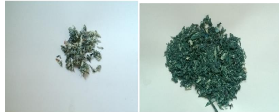
Figure 5. Products resulting from the shredding of Olyset Net type packaging.
