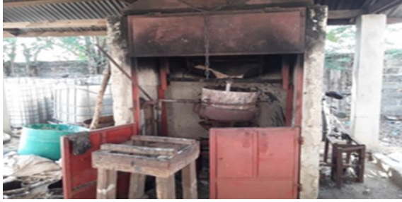
Figure 6. Handcrafted mixer used on the site.
