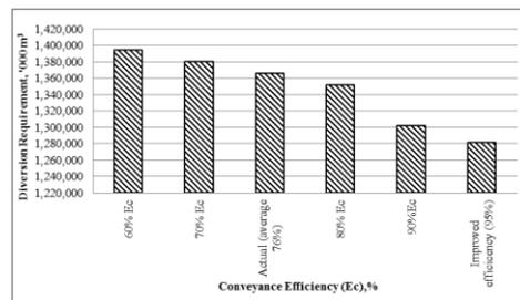
**Fig. 4.** Diversion requirement and conveyance efficiency. Note: Ec is the conveyance efficiency.
