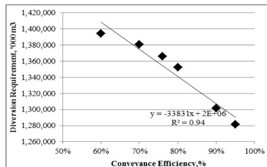
**Fig. 5.** Relationship of diversion requirement and conveyance efficiency.
