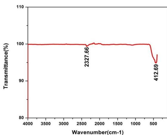
**Fig. 3.** FTIR image of Cerium oxide nanoparticles.
