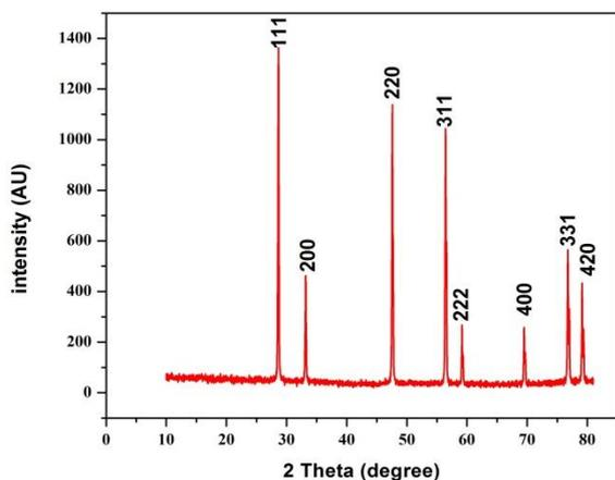
**Fig. 1.** XRD images of cerium oxide nanoparticles.
