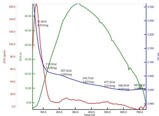
**Fig. 5.** TGA Curve of Cerium oxide nanoparticles.
