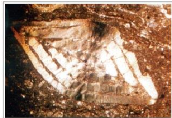
Fig. 4. 12. Photomicrograph of Wackestone biomicrite unit of Chorgali Formation (Sample No. CG 1-a ) showing meridian section of Nummulites mamillatus .
