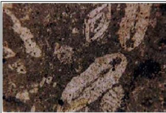
Fig. 4. 3. Photomicrograph of Wackestone-biomicroite unit of Margalla Hill Limestone (Sample No. C 19 ) showing Assilina sp. and Nummulites sp. in micrite cement (PPL. x2.5).
