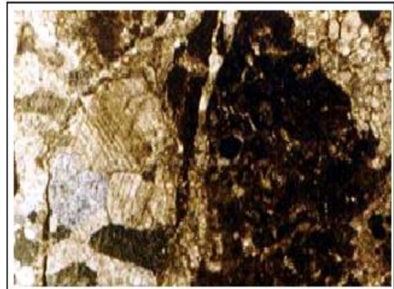
Fig. 4. 8. Photomicrograph of Wackestone dolomitic unit of Chorgali Formation (Sample No. Pd 2 ) showing calcite crystals, some pellets and dolospar crystals at upper right (Cross Nicol. x4).
