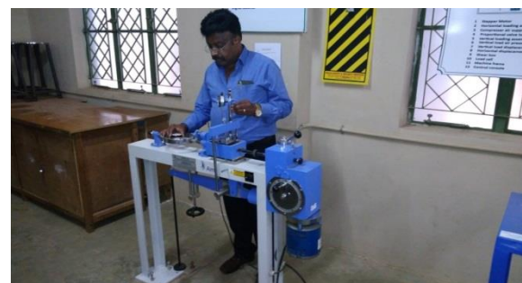
Fig. 5. Direct shear tests to determine shear parameters.
