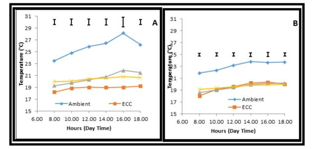
**Fig. 1.** Change in Temperature (°C) from morning to afternoon hours in Zero Energy Brick Cooler (ZEBC), Evaporative Charcoal Cooler (ECC), Pot-in-Pot, and ambient storage for Season 1 (A) and 2 (B). Top Bars represent LSD of means ( $P \le 0.05$ ).
