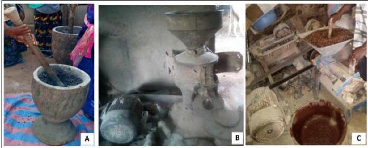
Fig. 1. Peeling equipment. A-Mortar and pestle, B-Abrasive wheel dehusser, C-Engelberg dehusser.
