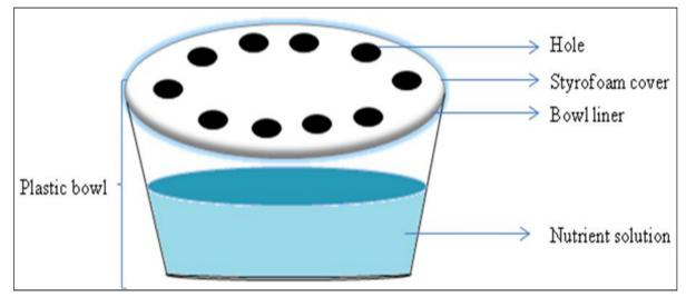
Fig. 1. Plastic bowl with Styrofoam cover.
