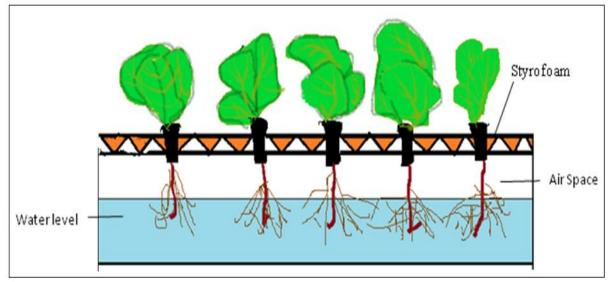
Fig. 2. Cross section of a non circulating hydroponic system.
