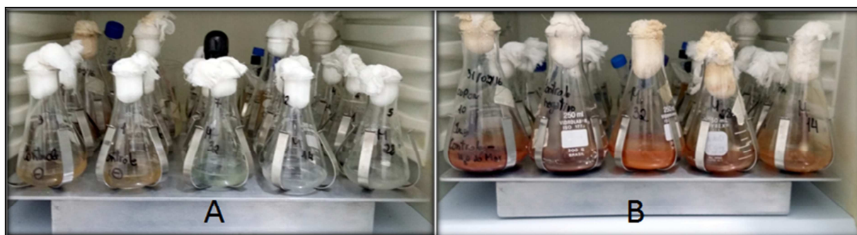
Fig. 2. Corrosion experiments in first day (A) and after 30 days (B), respectively.
