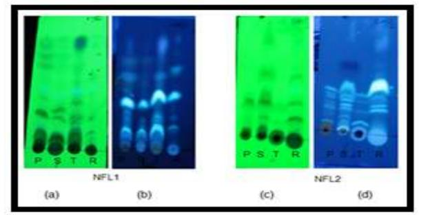
**Fig. 2.** TLC plates showing the detection of different compounds in crude extracts of NFL1 and NFL2 in order P=PDA, S=SDA, T=TM, R=Rice (a,b) Short (254nm) and Long UV (365nm) lightThin layer chromatogram of NFL1(c,d)Short and Long UV light Thin layer chromatogram of NFL2.
