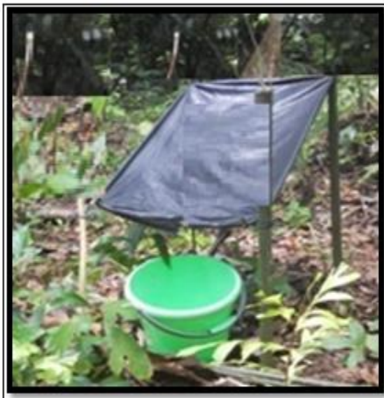
Fig.2. Measurement throughfall at study site. Based on the hydrological parameter, tree architectural model influences the value of runoff
