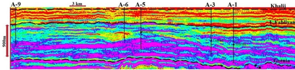
**Fig. 8.** A Northward trending inverted seismic section through wells A-6, A-5 illustrate a clear shelf break between the wells A-6, A-5, resulted in a lithofacies change which confirm by the well data (Fig. 7).
