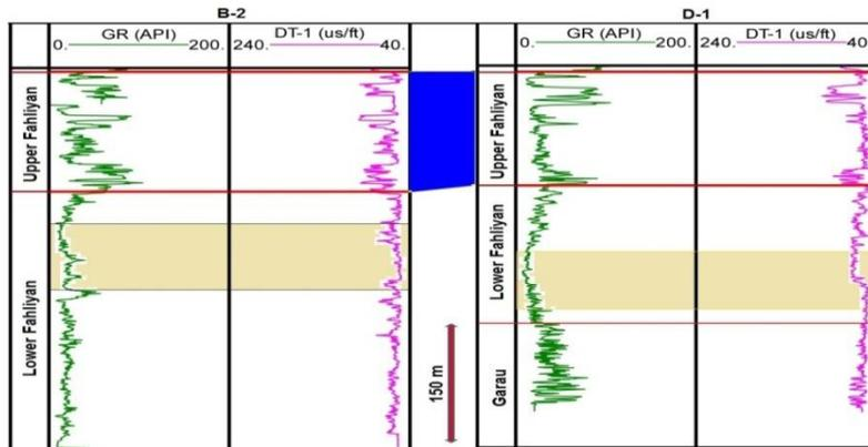
**Fig. 5.** Log correlation of Fahliyan Formation in a NE ward direction through wells B-2, D-1, a number of reservoir layers in well B-2 cannot be followed in D-1, due to facies change of the Fahliyan to Garau.
