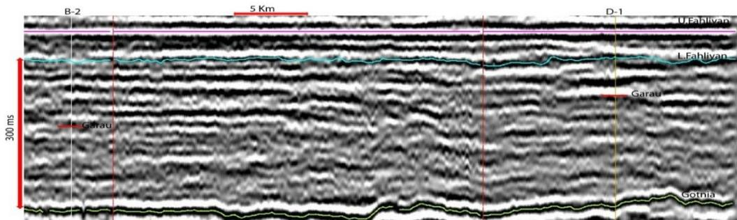
**Fig. 6.** A NE ward Seismic section through wells B-2 to D-1. Well B-2 located on the paleo-high, whereas well D-1 located down dip on the eastern flank of the paleo-high.
