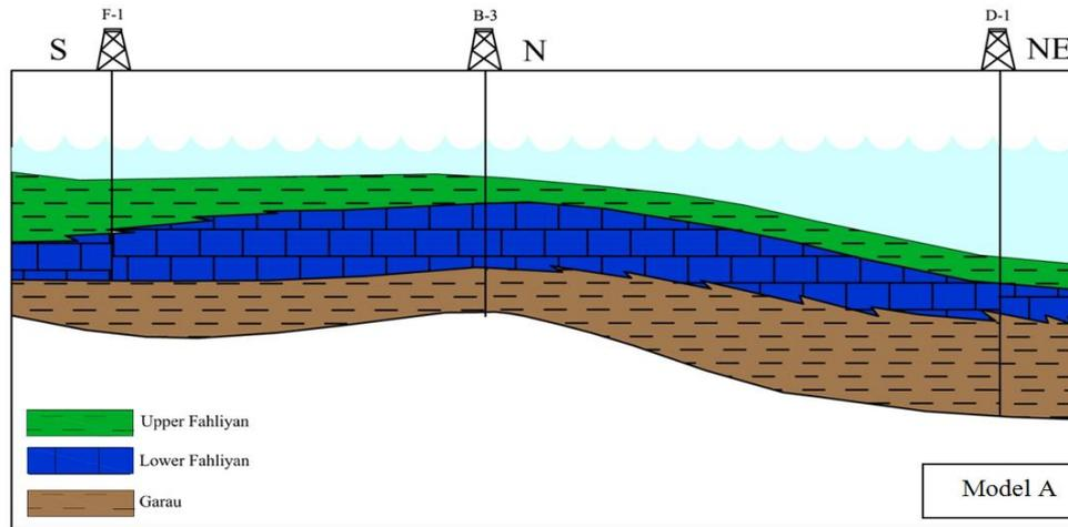
**Fig. 13.** A conceptual depositional model of Lower Cretaceous Garau, Upper and Lower Fahliyan formations in the most parts of the Abadan plain, based on the stratigraphic column of Wells F-1, B-3 and D-1.
