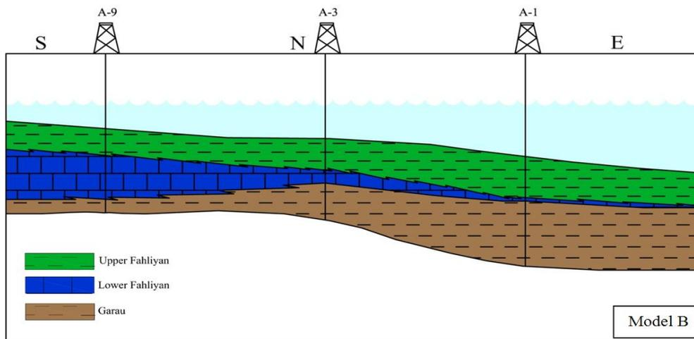
**Fig. 14.** An alternative conceptual depositional model of Lower Cretaceous Garau, Upper and Lower Fahliyan formations in the northern part of the Abadan plain, based on the stratigraphic column of Wells, A-9, A-3 and A-1.
