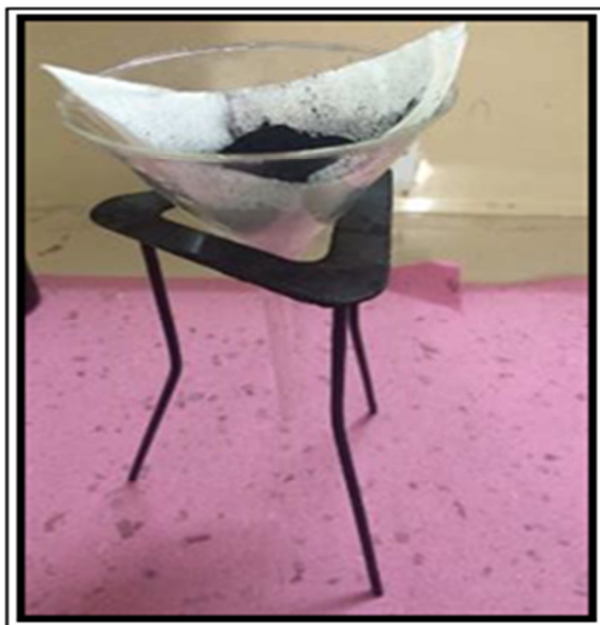
Fig. 2. Experimental set up for treatment of food color solutions with activated carbon.
