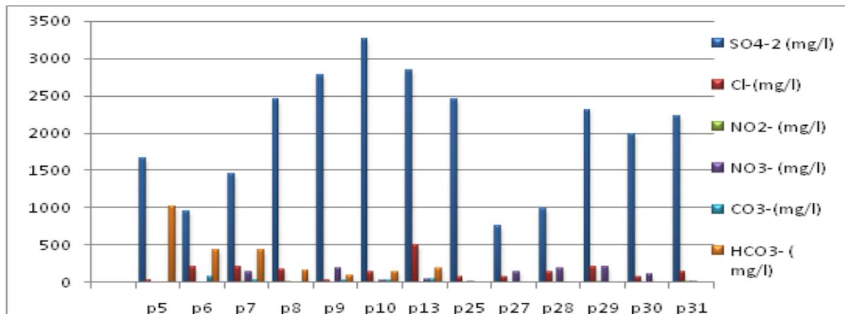
Fig. 6. The anion concentration of Groundwater.
