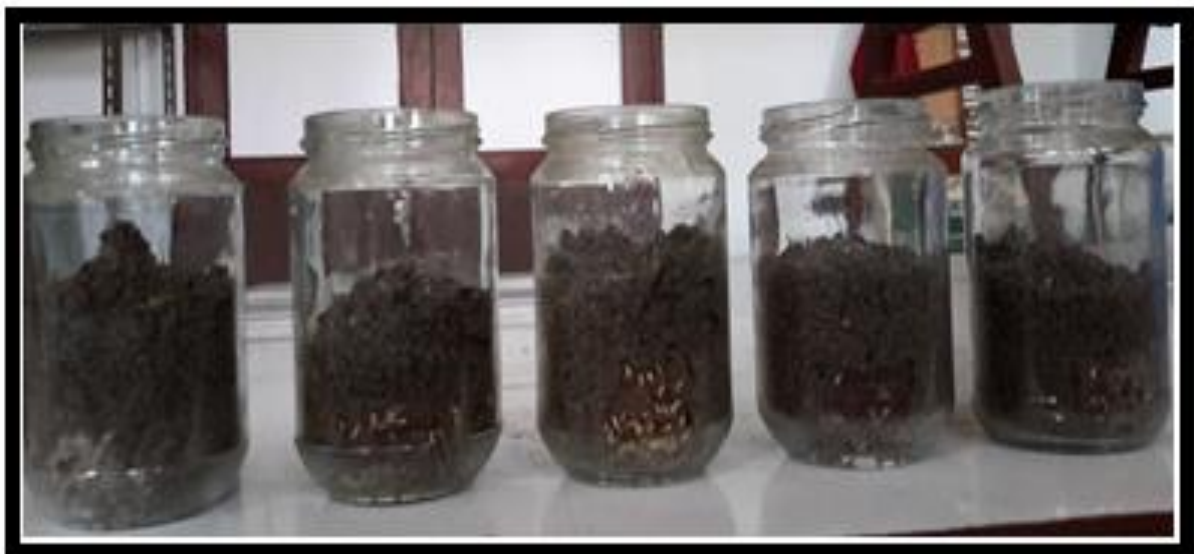
Fig. 2. Testing Wood Samples on Subterranean termites Attack for Four Weeks.
