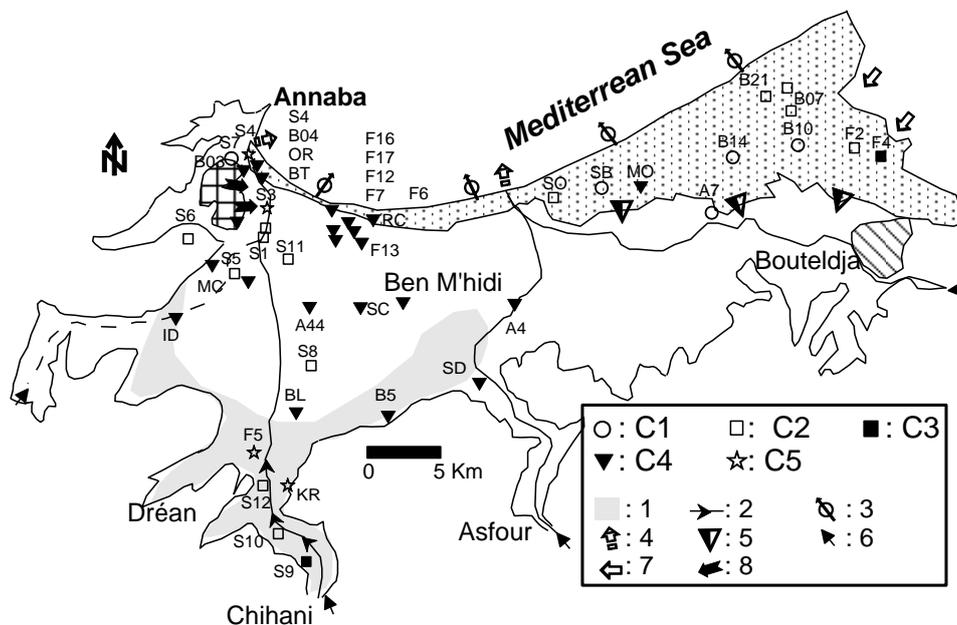
**Fig. 5.** Hydrogeology and major groundwater flow paths in the Annaba-Bouteldja region: (1) zone of weak thickness of the semi-permeable; (2) recharge zone of the aquifer; (3) groundwater toward the sea; (4) outflow toward the sea; (5) drainage of dune aquifer by the gravel aquifer; (6) contributions by rivers; (7) contributions from the Numidian rocks; (8) contributions from the metamorphic rocks.
