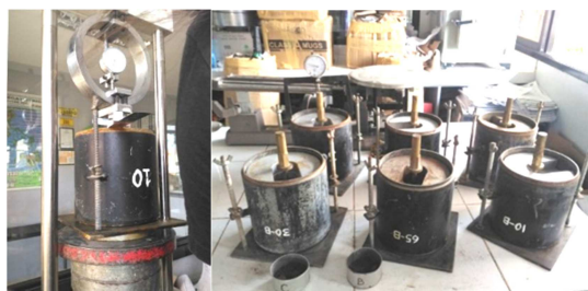
Fig. 1. California Bearing Ratio Test.
