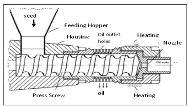
Fig. 1. Hole cylinder press of a KOMET oil expeller
