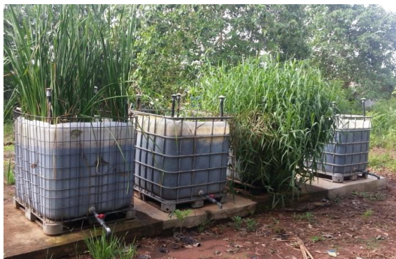
Picture 1. The planted filter pilot. Left to right: 1- Typha domingensis basin, 2- Panicum maximum basin, 3- Echinochloa pyramidalis basin and 4- Unplanted basin.
