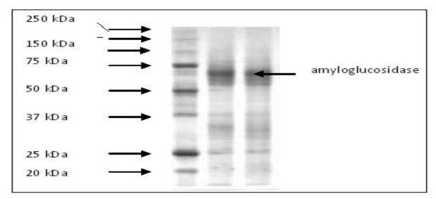
Fig. 1. SDS-PAGE of partially purified amyloglucosidase along with marker proteins.
