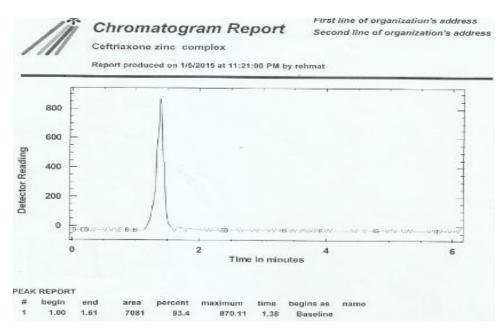
Fig. 10. HPLC chromatogram for Zinc ceftriaxone complex showing sharp peak and low retention time for zinc complex.
