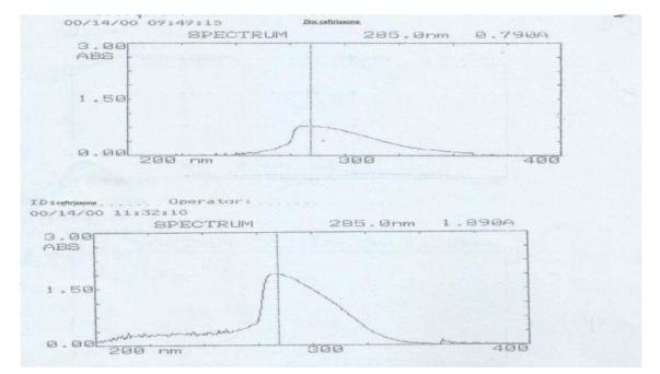
Fig. 7. UV spectra for ceftriaxone and zinc ceftriaxone chloride.
