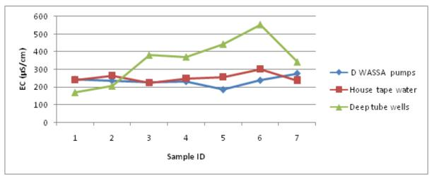
Fig. 4. Difference of Electrical conductivity in different water sources.
