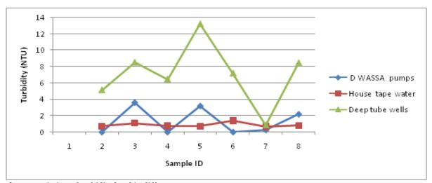
Fig. 3. Deviation of turbidity level in different water sources.
