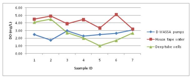
Fig. 5. Dissimilarity of DO level in different water sources.
