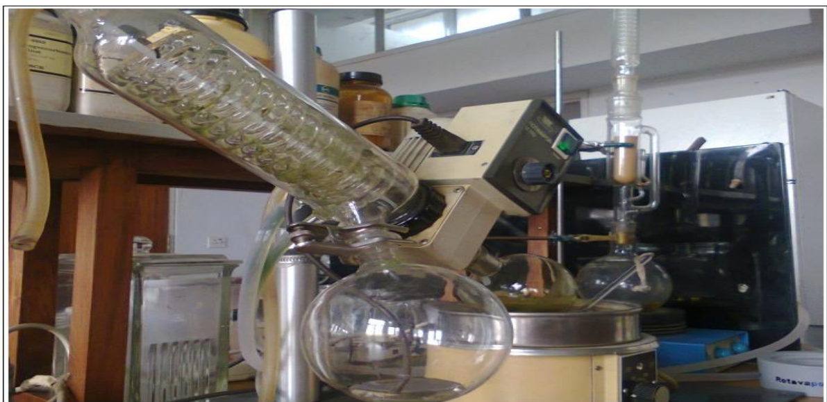
Fig. 7. Extract drying under reduced pressure.
