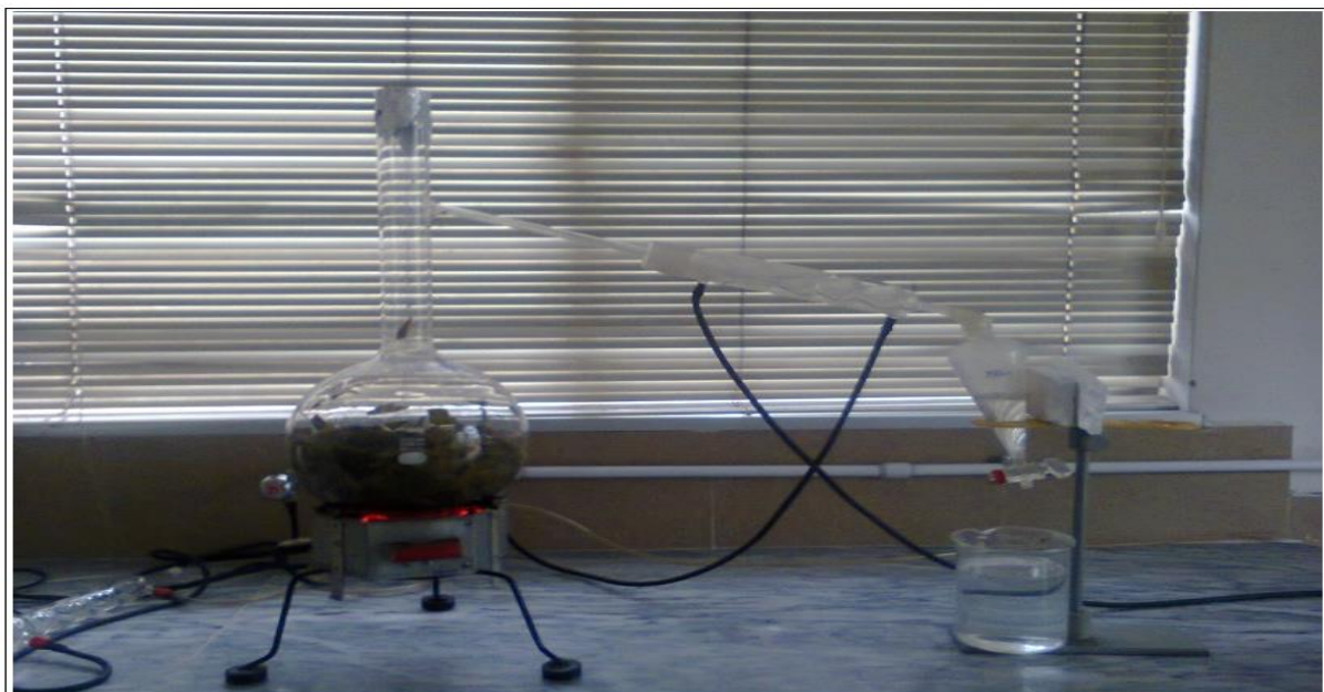
Fig. 3. Hydrodistillation of E.oil.
