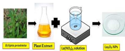
**Fig. 1.** Synthesis of Lanthanum oxide NPs.
