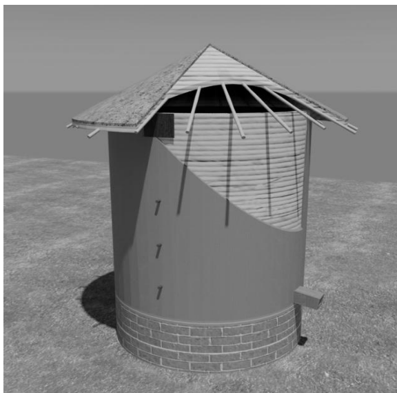
Fig. 2. Three dimensional view of the straw-clay bin.
