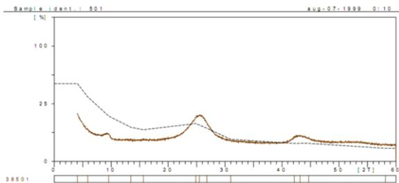
**Fig. 3.** XRD pattern of carbon nanotubes.
