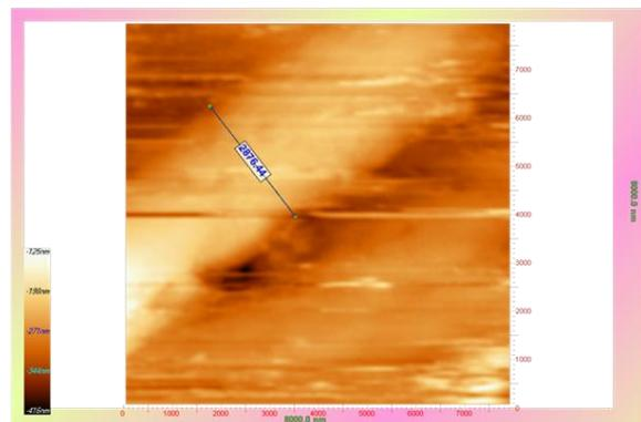
**Fig. 1.** Image of carbon nanotubes by STM.
