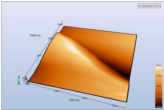
**Fig. 2.** Topographic image of carbon nanotubes by STM.
