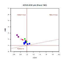
**Fig. 17.** Determination graph of saturation level of Alumina among Takestan rocks that are mostly categorized in meta-alumina range.
