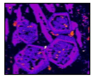
**Fig. 5.** Filtered X-ray picture that shows mixed zoning in garnet crystals.
