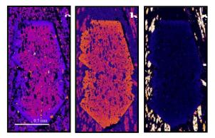
**Fig. 3.** Qualitative analysis pictures for Ca (a), Fe (b) and Mg (c) in a garnet crystal with normal zoning.
