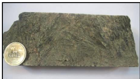
Fig. 3. Host rock of macro crystal, with relatively homogenous texture that locates actinolites besides magnetite.
