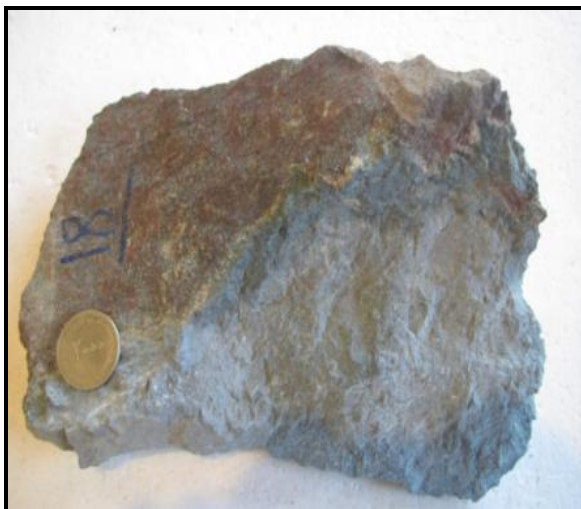
Fig. 5. A rock sample from far region of mineralization, magnetite signs are not observable in these rocks.
