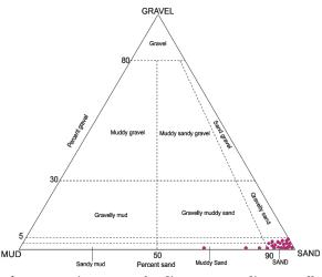
**Fig. 5.** Naming types of sediments according to Folk method.
