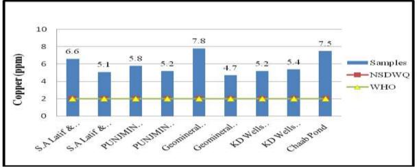
Fig. 7. Copper Concentration in samples along with the standard values.
