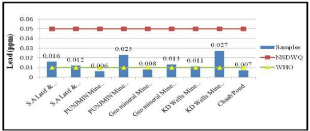
Fig. 8. Lead Concentration in samples along with the standard values.
