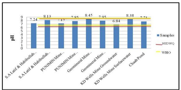
Fig. 4. Comparison of pH of samples with standards.
