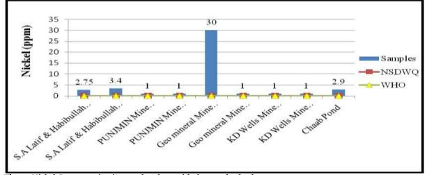
Fig. 9. Nickel Concentration in samples along with the standard values.
