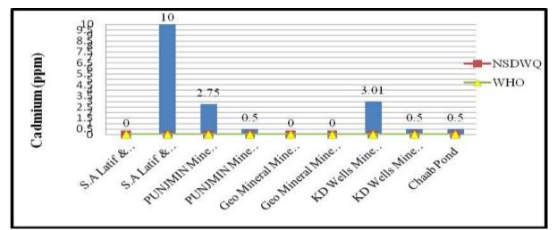
Fig. 6. Cadmium Concentration in samples along with the standard values.
