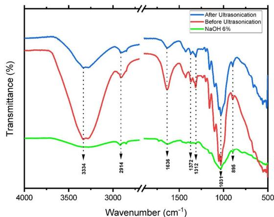
**Fig. 2.** FTIR spectra of 6% NaOH alkalinized water chestnut fiber and microfibers before and after ultrasonication.
