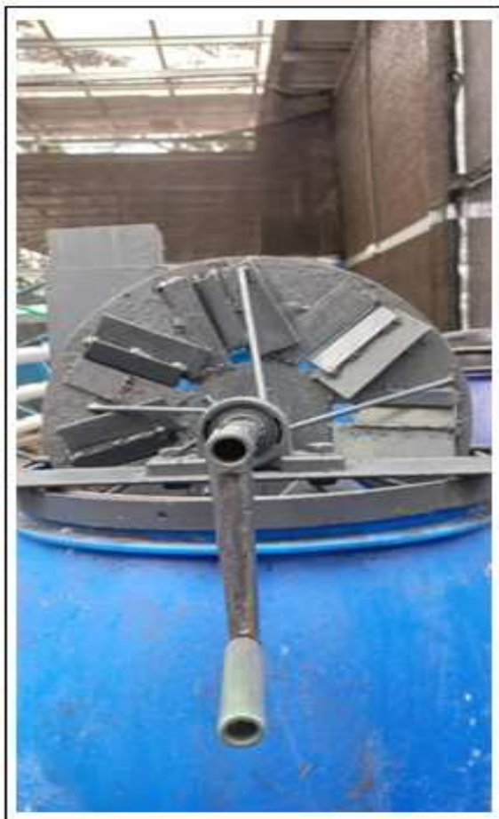
Fig. 4. Compost Bin with a Chopper.
