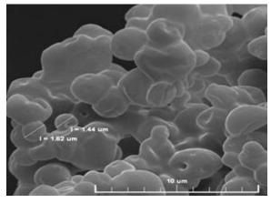
**Fig. 9.** Scanning electron microscope (SEM) of encapsulated fish oil powders prepared with 15% Inilin & 5% Casein.
