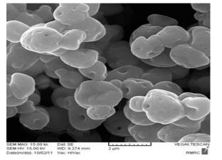
Fig. 7. Scanning electron microscope (SEM) of encapsulated fish oil powders prepared with 20% Inilin.
