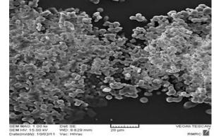
**Fig. 8.** Scanning electron microscope (SEM) of encapsulated fish oil powders prepared with 10% Inilin & 10% Casein.
