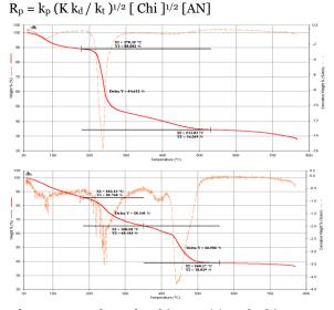
**Fig. 2.** TGA of crude Chitosan (a) and Chitosan-g-PolyAN (b).
