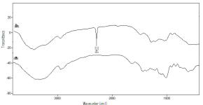
**Fig. 1.** FTIR spectra of (a) crude Chitosan and (b) homopolymer-free Chitosan *-g*-PolyAN. *Reaction rate*
