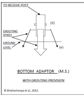
**Fig. 2.** Elevation of bottom grouting part of the adjustable trap (For labels see text)
