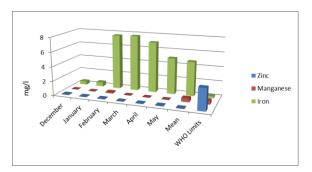
**Fig. 2.** Showing concentration of Zinc, Mn and Fe in surface water samples of River Panjkora.
