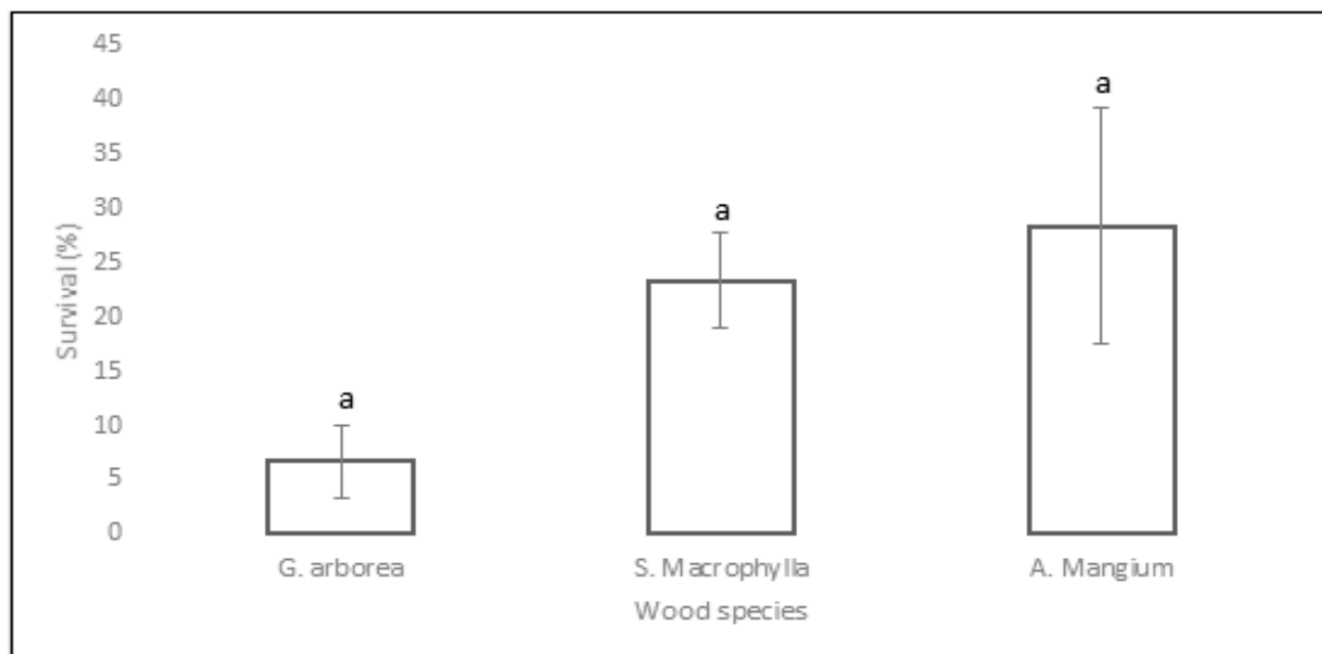
Fig. 2. Survival (%) of termite (mean ± SEM) after 119 days of no-choice feeding test Means followed by the same letter are not significantly different (Tukey's HSD: p < 0.05 ).
