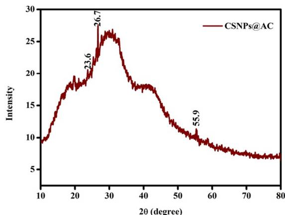
**Fig. 1.** The XRD graph of Chitosan nanoparticle doped Activated Carbon (CSNPs@AC).
