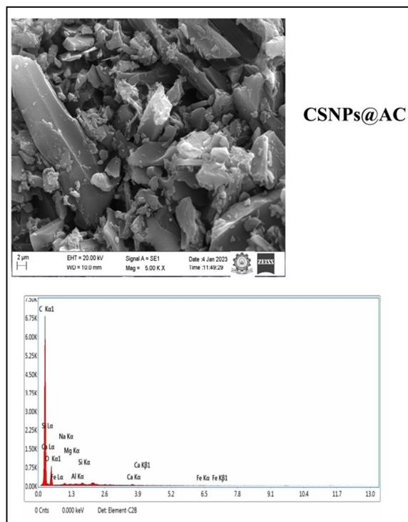
**Fig. 3.** The SEM-EDX graph of Chitosan nanoparticle doped Activated Carbon (CSNPs@AC).
