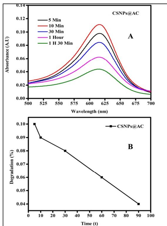
**Fig. 5.** The Photocatalytic graph of Chitosan nanoparticle doped Activated Carbon (CSNPs@AC) (a) represents Chitosan nanoparticle doped Activated Carbon (CSNPs@AC) (b) represents the degradation of dye from Chitosan nanoparticle doped Activated Carbon (CSNPs@AC).
