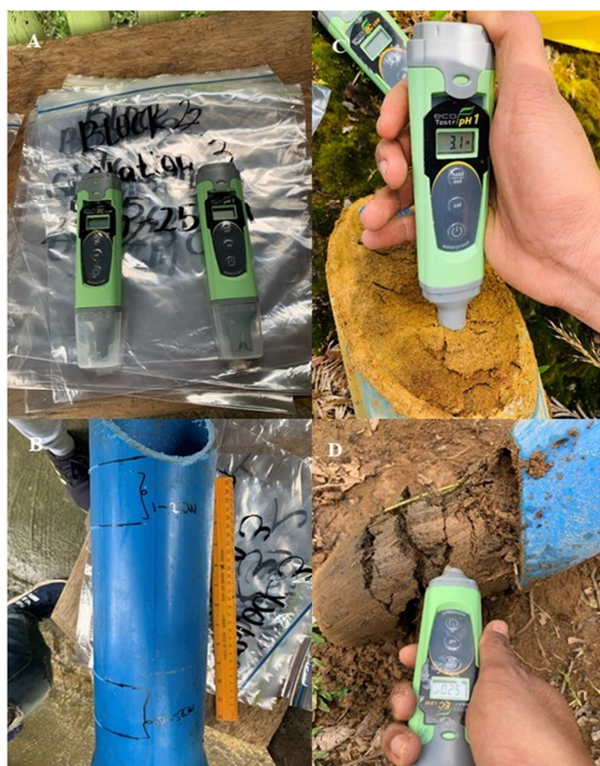
Fig. 2. A-B, Apparatus used to determine the pH and electro conductivity of the soil samples and improvised soil auger during sampling. C-D, Soil testing for pH and EC from two soil depths.
