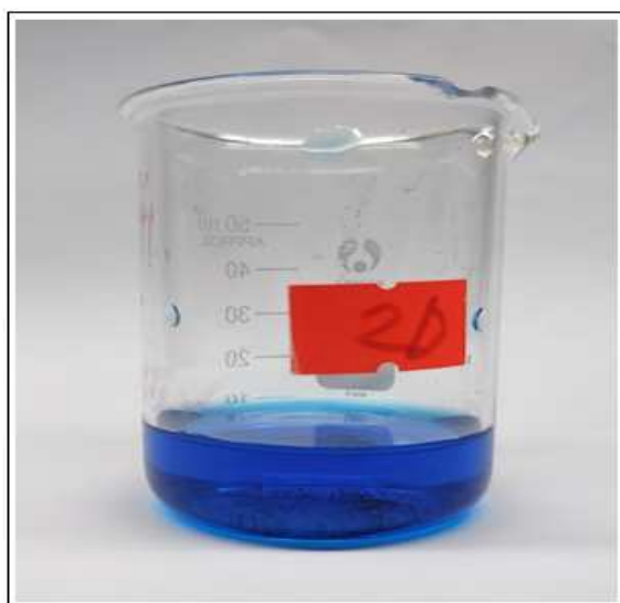
Fig. 1. 10ml MB solution (10mg/L) with 10% H 2 O 2 and 4mg/L MNPs.
