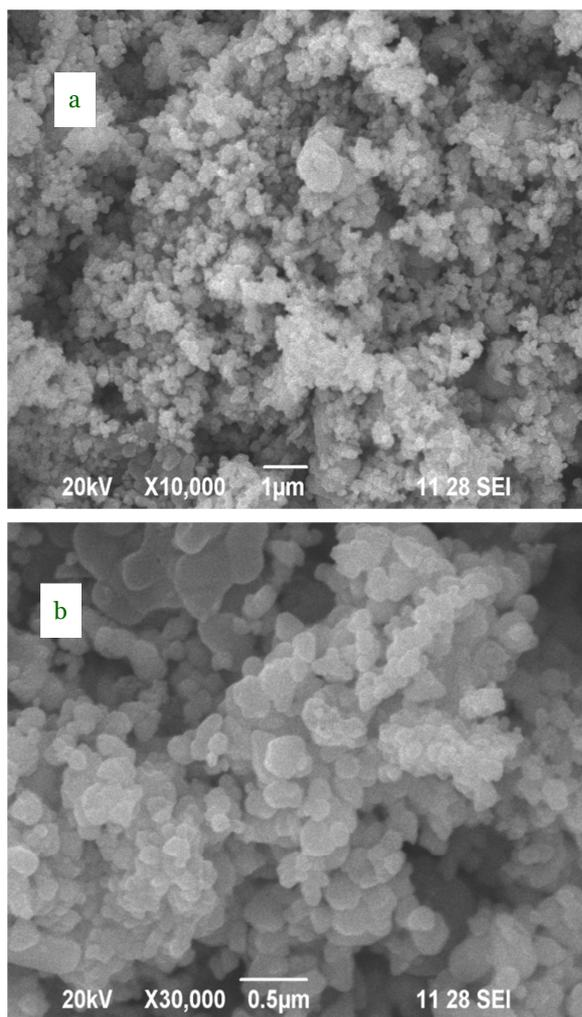
**Fig. 2.** The structural morphology of the synthesized a. ZnO/ SA nanocomposite and b. ZnO /cmC nanocomposite
