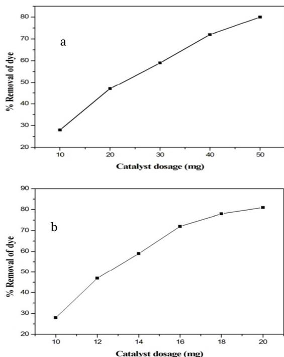
**Fig. 9.** Variation of % removal of the dye against catalyst loading for a.ZnO / SA and b. ZnO /cmC.
