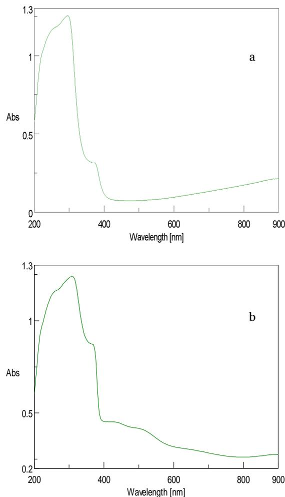
**Fig.** UV-Vis absorption spectra of a.ZnO / SA b. ZnO /cmC nanocomposite
