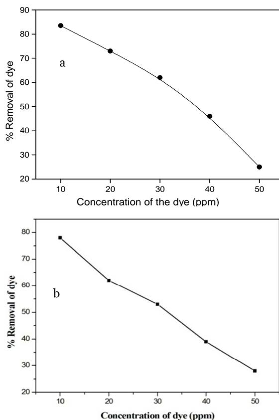
**Fig. 10.** Variation of% removal of the dye against concentration of the dye for a.ZnO /SA and b. ZnO /cmC
