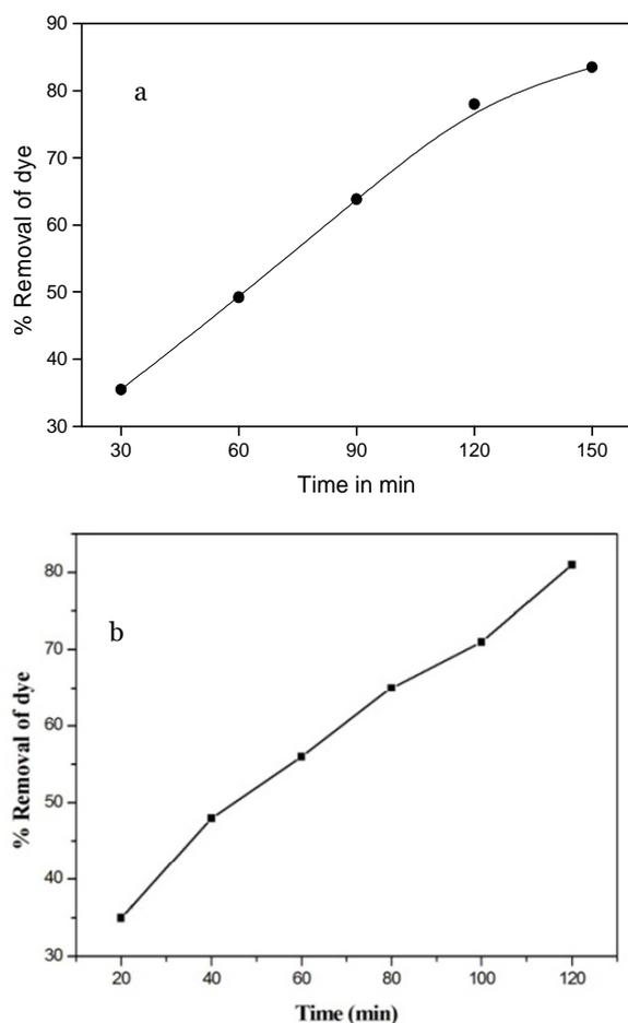
**Fig. 11.** Variation of% removal of MB dye against irradiation time for a.ZnO / SA and b. ZnO /cmC.
