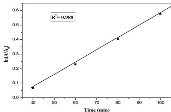
**Fig. 8.** The photocatalytic degradation of MB dye and kinetics fit for the degradation..
