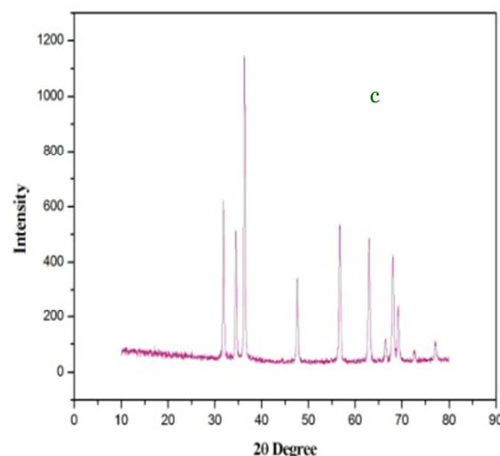
**Fig. 1.** The XRD patterns of a. precursor ZnO b. ZnO/SA c. ZnO/cmC.
