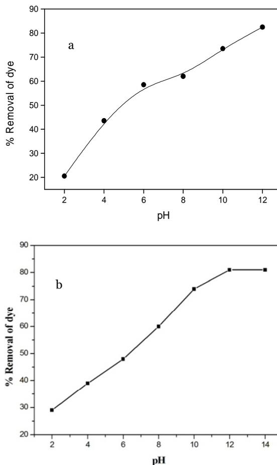
**Fig.12.** Variation of% removal of MB against pH for a.ZnO / SA and b. ZnO /cmC.
