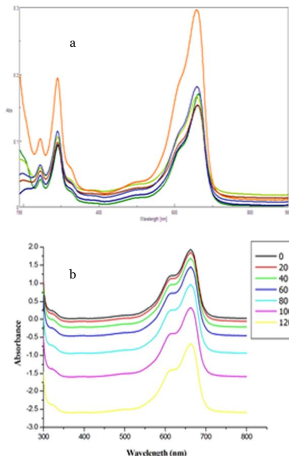
**Fig.7.** UV-Vis spectra of MB dye treated under photocatalytic reaction in the presence of a. ZnO / SA and b. ZnO /cmC.
