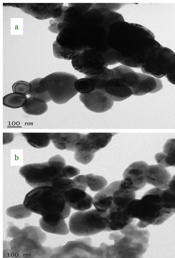
**Fig. 3.** The TEM image of the prepared a. ZnO/ SA and b. ZnO /cmC nanocomposite
