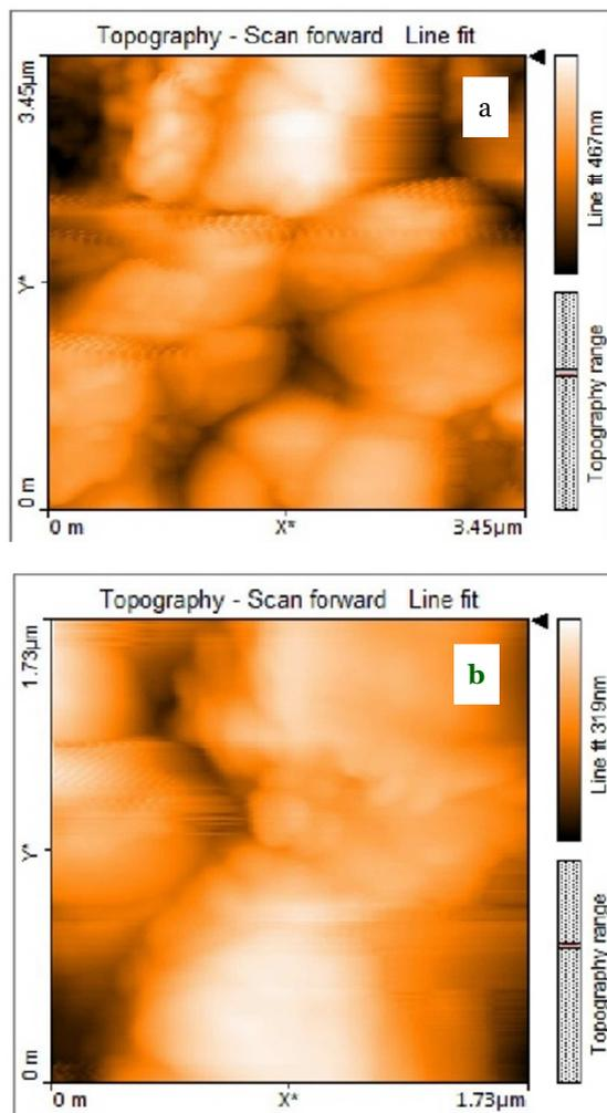
**Fig. 6.** AFM images of a. ZnO / SA b. ZnO /cmC.
