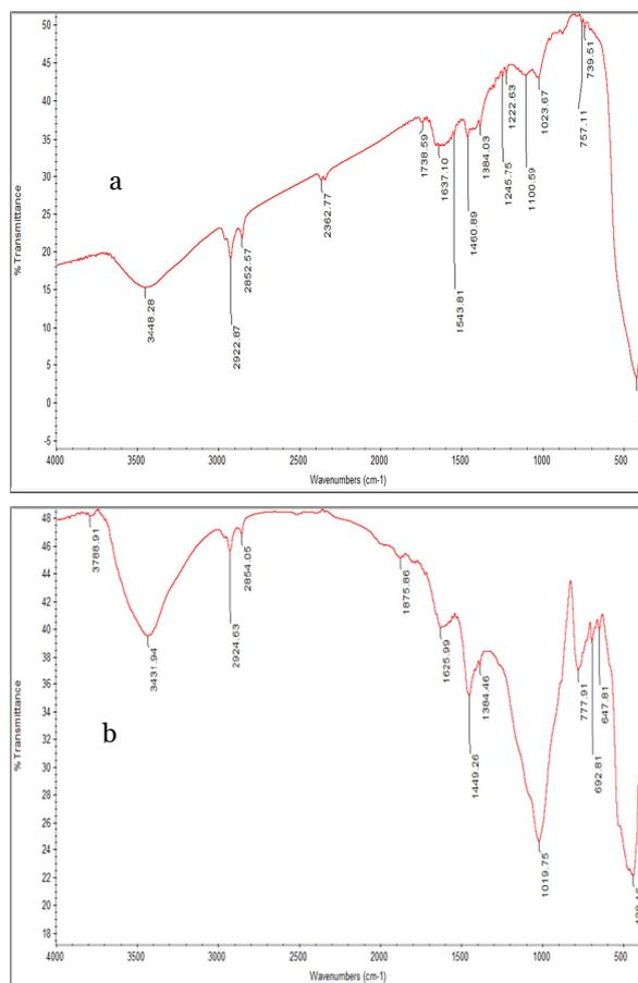
**Fig. 4.** Fourier transform infrared spectroscopy (FTIR) data of the a. ZnO/ SA and b. ZnO /cmC nanocomposite
